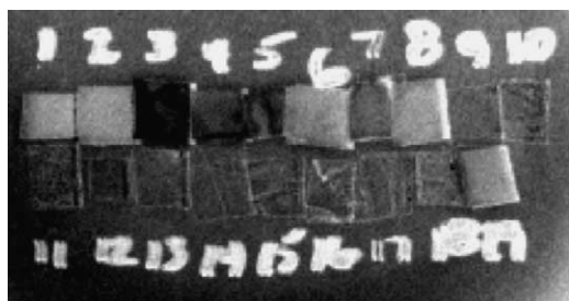
Fig. 5. Macroscopic colour chemical imaging of tape backings (extracted at 400 nm).
